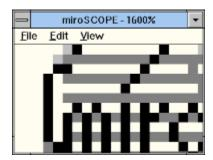
If you move the cursor out of the miroSCOPE window, the miroSCOPE window shows the current cursor position. If the cursor is moved within the miroSCOPE window, the mouse cursor changes its shape and becomes a magnifying glass. Clicking the left mouse key magnifies the window content, clicking the right mouse key makes the windows contents smaller.
